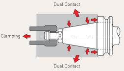
Taper Dual Contact Spindle
